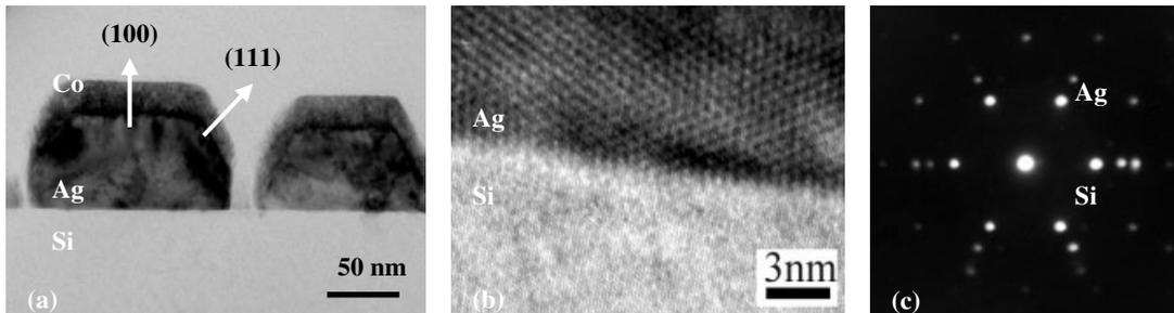
**Fig. 2** Cross-sectional TEM micrograph of the Co films grown on Si(111) substrate with 60 nm thick Ag buffer (a); (b) is HRTEM morphology of Si/Ag interface, and (c) is the electron diffraction pattern corresponding to (b).
