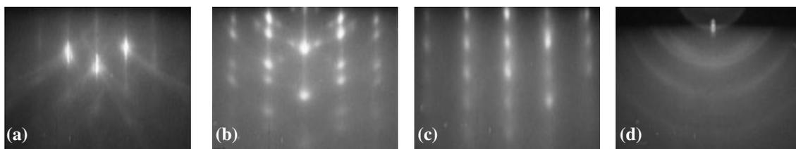
**Fig. 1** RHEED patterns of Si/Ag/Co films with the probing e-beam aligned along the Si[100] in-plane direction; (a) is for Si(111) substrate, (b) is with 5 nm thick Ag buffer on (a), (c) and (d) are RHEED patterns for Co (5 nm) films grown on (b) and (a), respectively.
