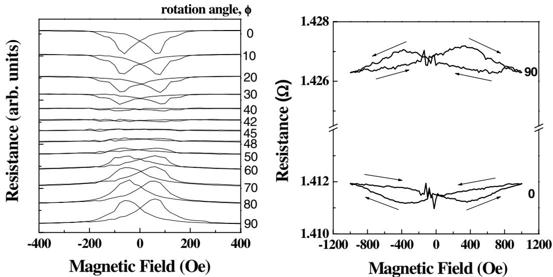
**Fig. 4** MR loops for the Co films grown on Si(111) substrates (a) without, and (b) with 20 nm thick Ag buffer layer. The rotation angle  $\phi$  is between the direction of the current and the orientation of the applied magnetic field.
