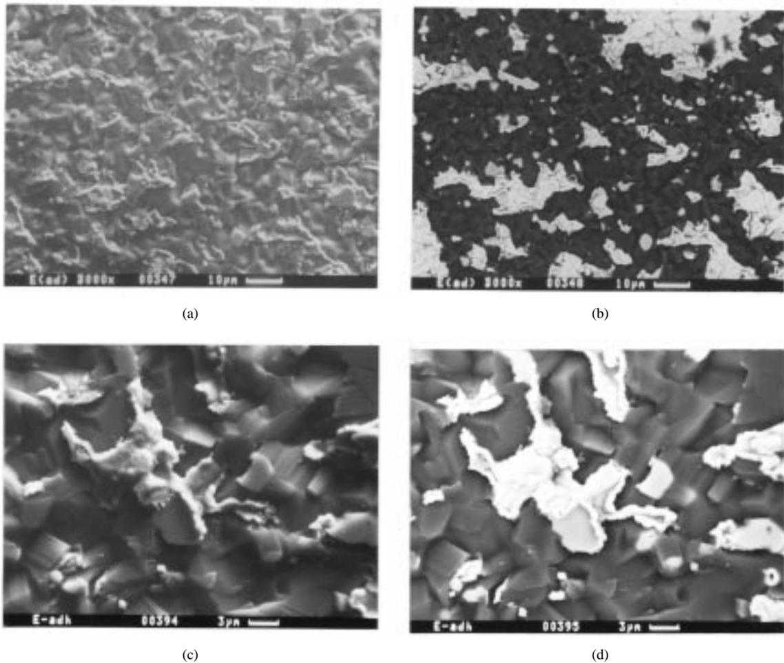
Fig. 10. Fractured surface of the EN-plated etched AlN substrate after pulling-off. (a) SEI micrograph, (b) corresponding BEI of (a), and (c) and (d) higher magnification pictures of (a) and (b), respectively. Large areas of the residual EN films are visible around the Al-Y-O compounds and irregular in shape.
