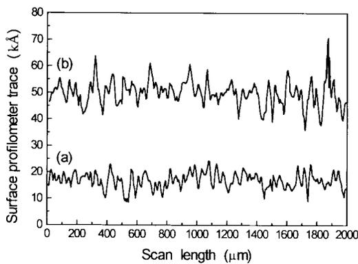
Fig. 3. The surface profilometer traces of the: (a) as-received AlN substrate and (b) EN film plating for 10 min.
