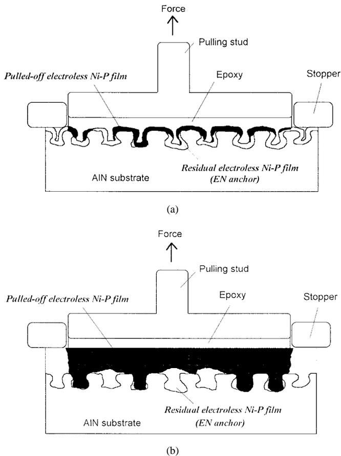
Fig. 16. Schematic diagrams to show the fracture mechanisms of the EN-plated AlN substrates under the pull-off testing for samples: (a) E and (b) T, respectively.
