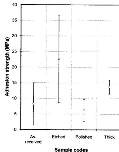
Fig. 6. Adhesion strength of samples A (as-received), P (polished), E (etched), and T (thicker EN film).
