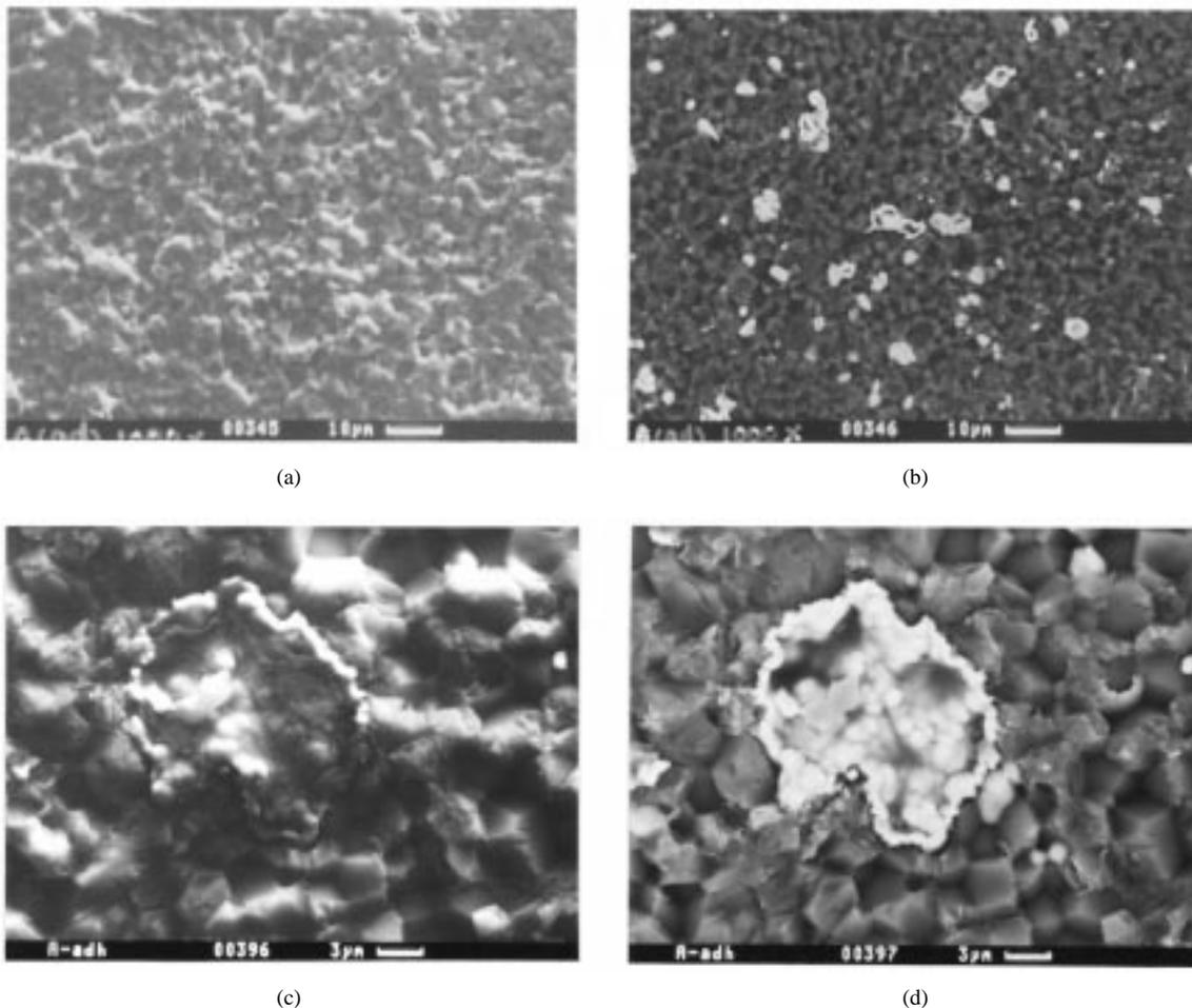
Fig. 11. Fractured surface of the EN-plated as-received AlN substrate after pulling-off: (a) SEI micrograph, (b) corresponding BEI of (a), and (c) and (d) higher magnification pictures of (a) and (b), respectively. A few residual EN films are left on the AlN fracture surface and exhibit round shapes.
