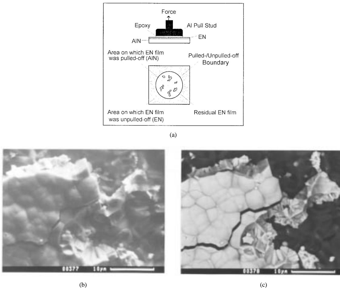
Fig. 15. The boundary between the pulled-off and unpulled-off areas in EN film. Cracks inside the unpulled-off EN film are mainly propagating along the particle boundaries: (a) Schematic diagram, (b) SEI micrograph and (c) BEI micrograph.
