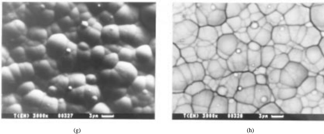
Fig. 2. (Continued.) Surface morphologies and corresponding BEIs of electroless Ni-plated AlN substrates for (g) and (h) thicker EN film on etched AlN substrate, respectively.
