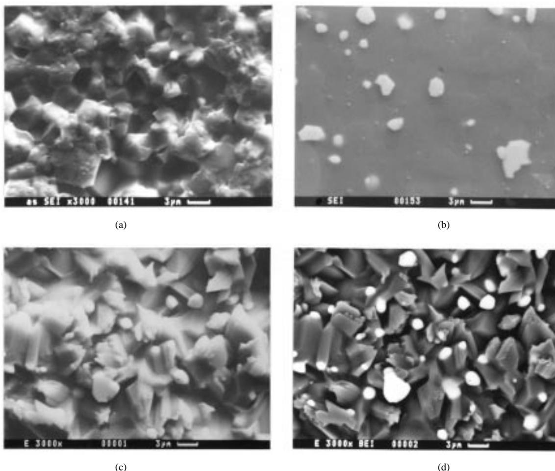
Fig. 1. Surface morphologies of: (a) as-received, (b) polished, (c) etched AlN substrate, and (d) corresponding BEI of (c).
