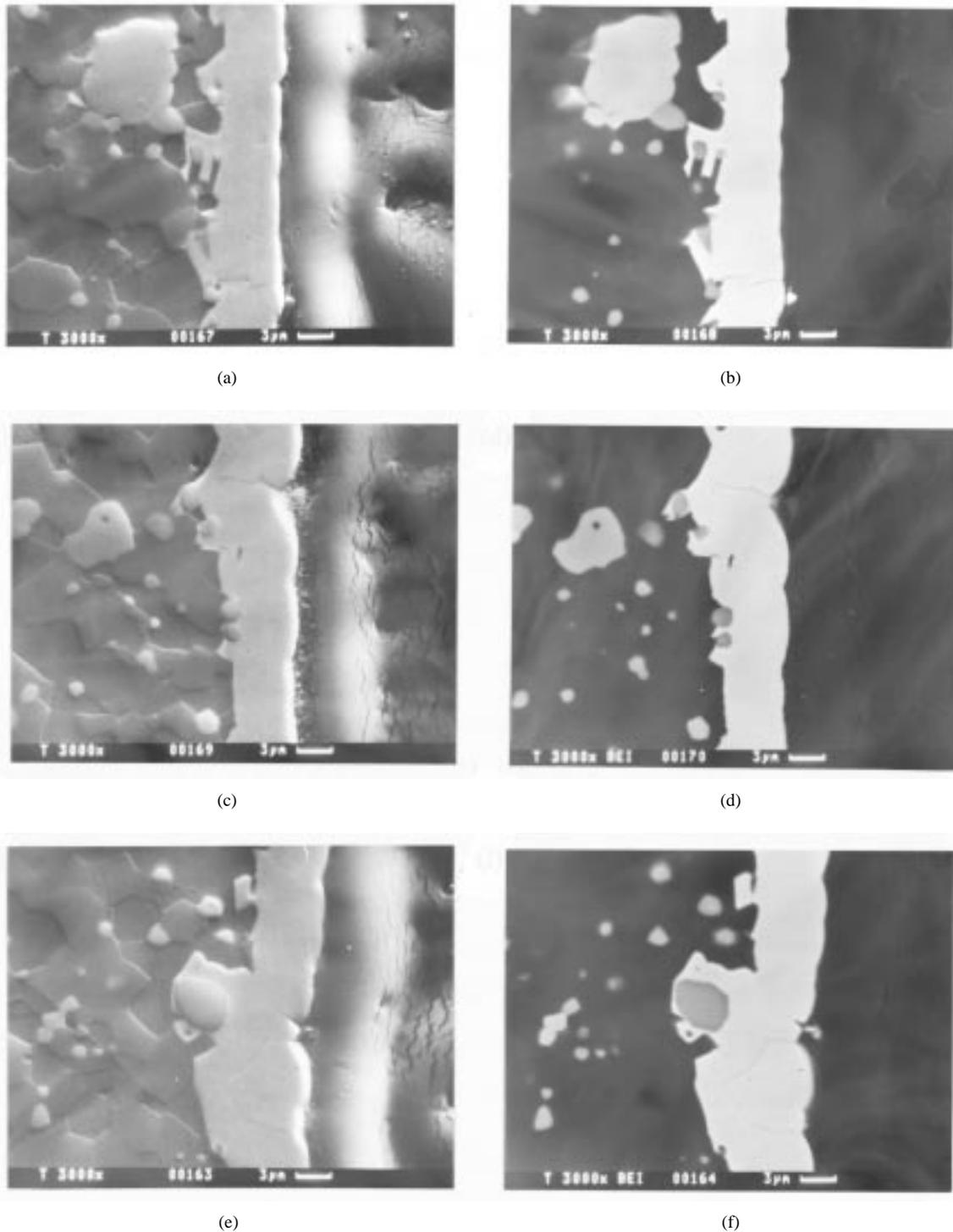
Fig. 13. Morphologies of the cross-sectional views of the thick EN films on the etched AlN substrates: (a), (c), (e), (g), (i), and (k) SEI micrographs, and (b), (d), (f), (h), (j), and (l) corresponding BEI of (a), (c), (e), (g), (i), and (k), respectively.
