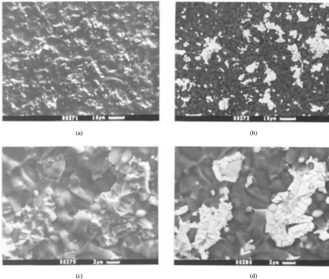
Fig. 14. Fractured surface of the etched AlN substrate with thick EN film plated on the EN film after pulling off test: (a) SEI micrograph, (b) corresponding BEI of (a), and (c) and (d) higher magnification pictures of (a) and (b), respectively.
