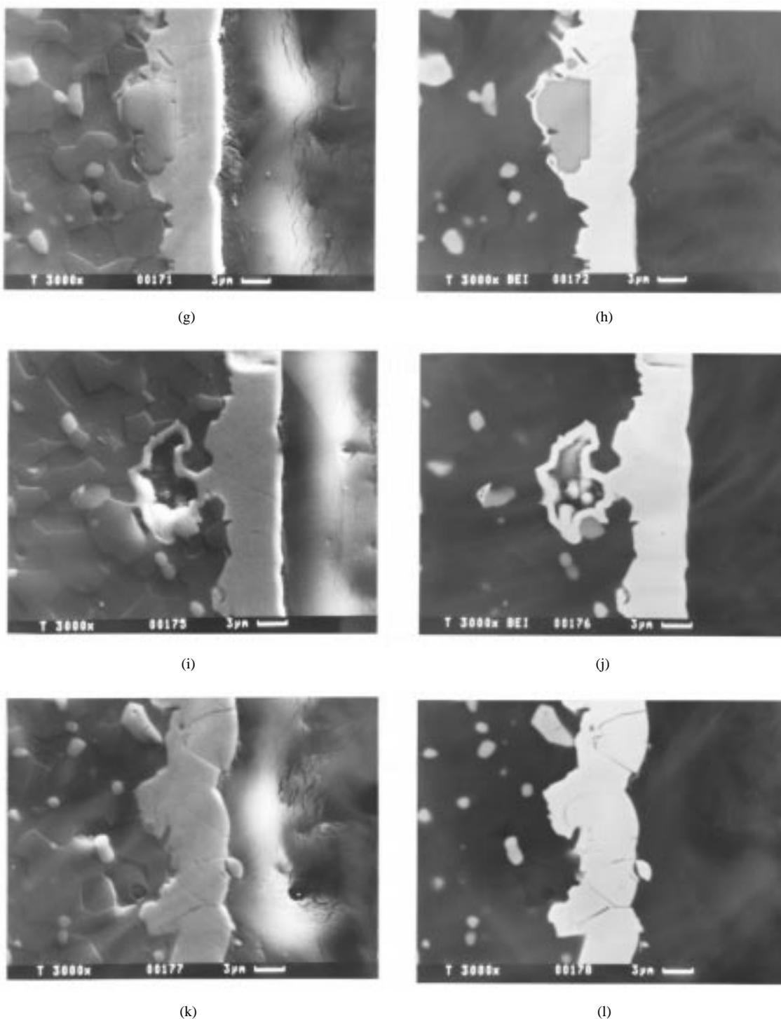
Fig. 13. (Continued.) Morphologies of the cross-sectional views of the thick EN films on the etched AlN substrates: (a), (c), (e), (g), (i), and (k) SEI micrographs, and (b), (d), (f), (h), (j), and (l) corresponding BEI of (a), (c), (e), (g), (i), and (k), respectively.
