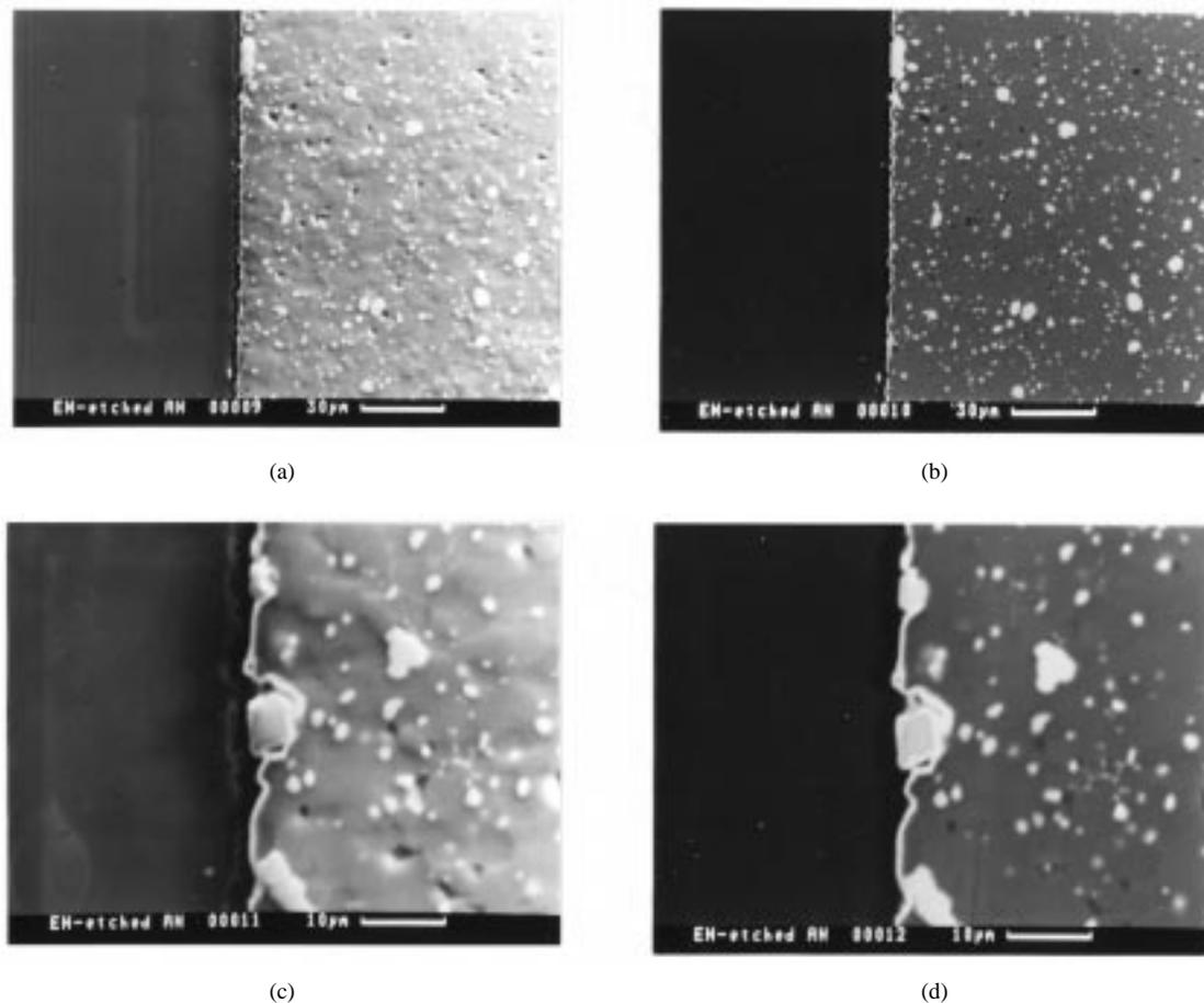
Fig. 7. Cross-sectional view of the EN film on the etched AlN substrate: (a) SEI micrograph, (b) corresponding BEI of (a), and (c) and (d) higher magnification pictures of (a) and (b), respectively. The EN film well contours AlN and penetrates into AlN surface around Al-Y-O compounds to form anchors.
