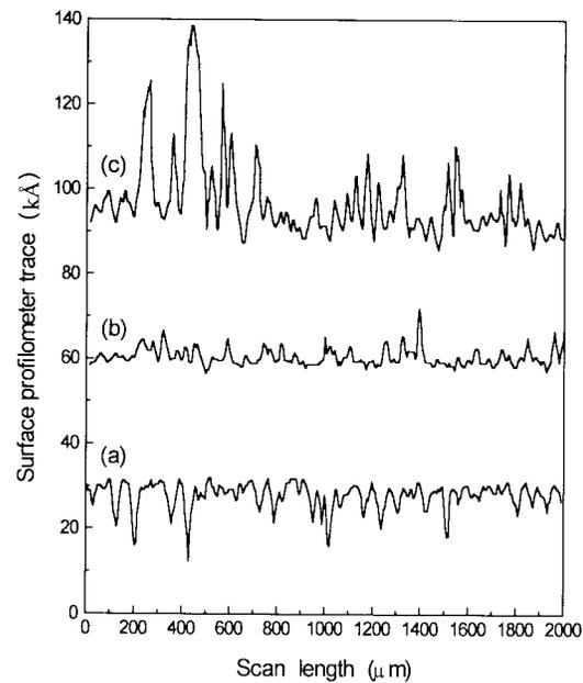
Fig. 5. The surface profilometer traces of the: (a) etched AlN substrate, (b) EN film plating for 10 min and (c) EN film plating for 2 h.
