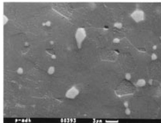
Fig. 12. Fractured surfaces of the EN-plated polished AlN substrates after pulling-off. No residual EN film is visible on the AlN fracture surface.
