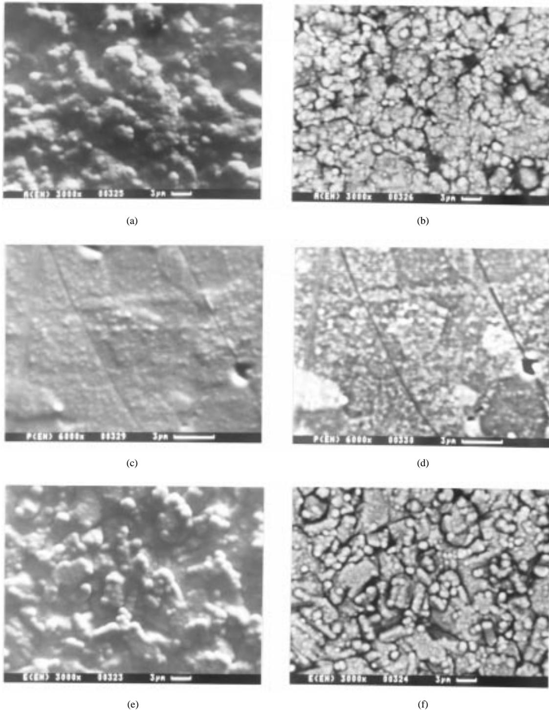
Fig. 2. Surface morphologies and corresponding BEIs of electroless Ni-plated AlN substrates for (a) and (b) as-received, (c) and (d) polished, (e) and (f) etched AlN substrates.
