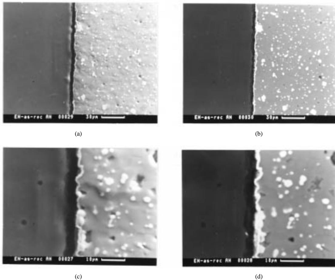
Fig. 8. Cross-sectional view of the EN film on the as-received AlN substrate. (a) SEI micrograph, (b) corresponding BEI of (a), and (c) and (d) higher magnification pictures of (a) and (b), respectively. The EN film well contours the rough AlN, but no apparent anchors are formed.
