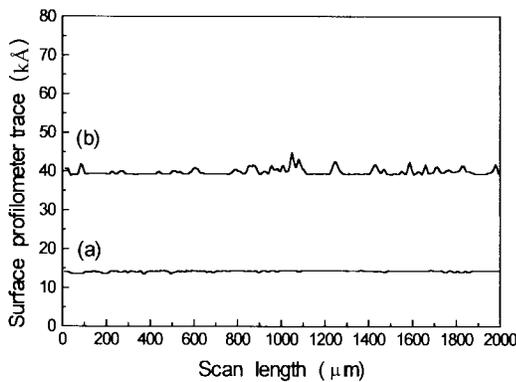
Fig. 4. The surface profilometer traces of the: (a) polished AlN substrate and (b) EN film plating for 10 min.
