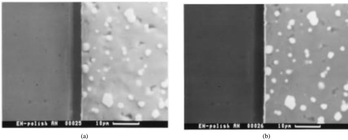
Fig. 9. Cross-sectional view of the EN film on the polished AlN substrate. (a) SEI micrograph, (b) corresponding BEI of (a). The EN film well contours the smooth AlN substrates and no anchors are formed.
