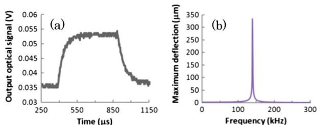
Fig. 5. (Color online) (a) Measured dynamic response of the modulated optical signal, (b) simulated frequency response of a 150- $\mu\text{m}$ -long suspended silicon waveguide.
