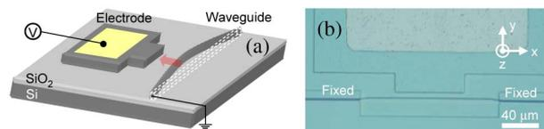
Fig. 1. (Color online) (a) Schematic of a MEMS-actuated phase modulation unit consisting of a deformable waveguide and an electrode, (b) top-view micrograph of a fabricated phase modulation unit.
