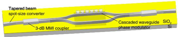
Fig. 3. (Color online) Schematic of a MEMS-actuated MZI.
