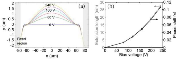
Fig. 2. (Color online) (a) Simulated waveguide deformation at different bias voltages, (b) calculated waveguide extension and the corresponding phase shift as functions of bias voltage.
