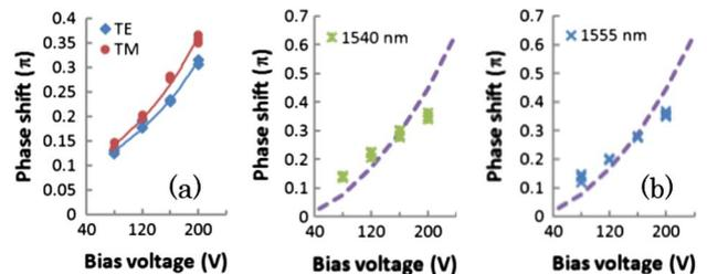
Fig. 4. (Color online) Experimental results on phase modulation. (a) Measured phase shifts as functions of bias voltages for the TE- and TM-polarized waves, (b) measured phase shifts at the wavelengths of 1540 and 1555 nm for the TM-polarized wave. The theoretical curves (dashed line) are calculated by the finite element method.
