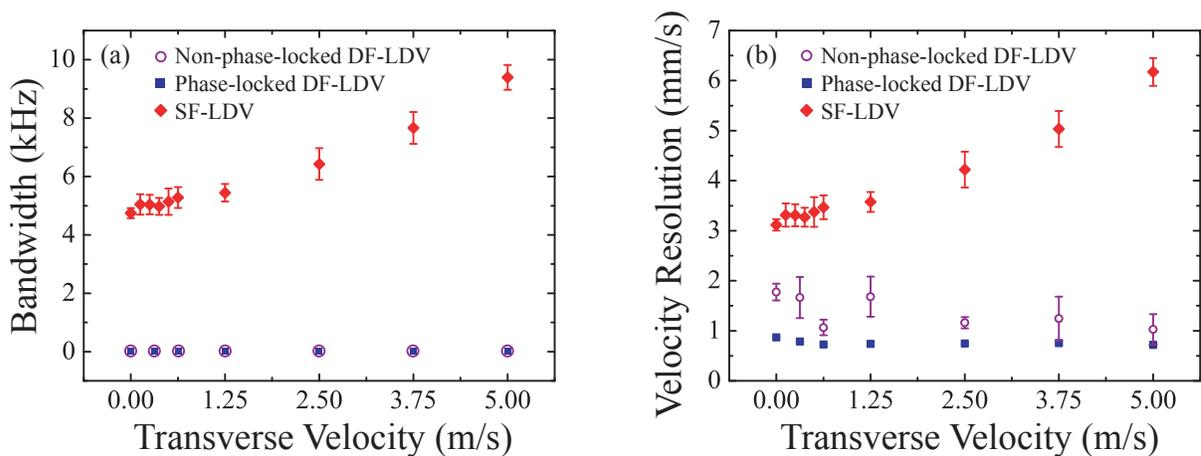
**Figure 3.** (a) -6 dB Doppler bandwidth measured from the received Doppler signals under different transverse velocities. (b) Velocity resolution under different transverse velocities.
