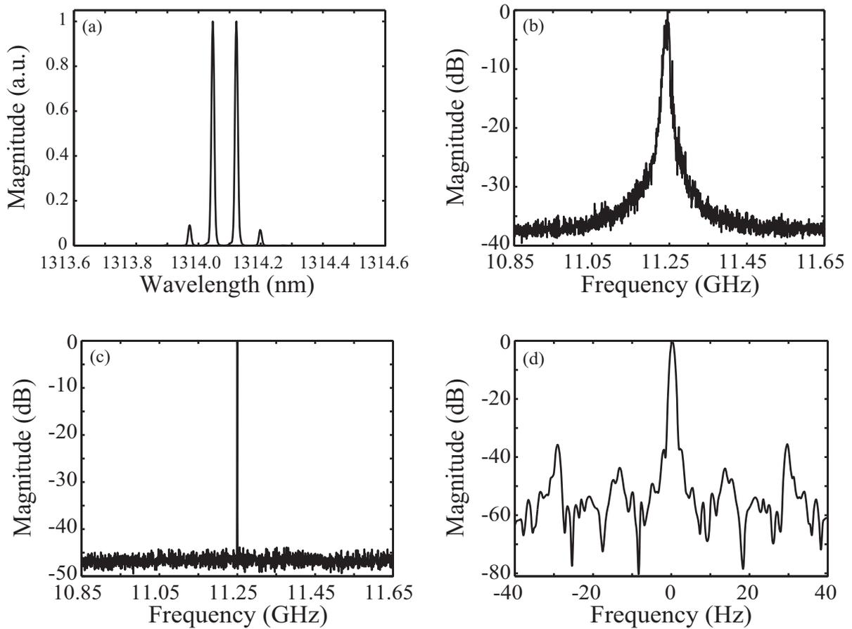
**Figure 2.** (a) The optical spectrum of the P1 dynamic state. (b) and (c) The corresponding electrical power spectra without and with the phase-lock technique. (d) The enlargement of (c) with the frequency axis offset to 11.25 GHz.
