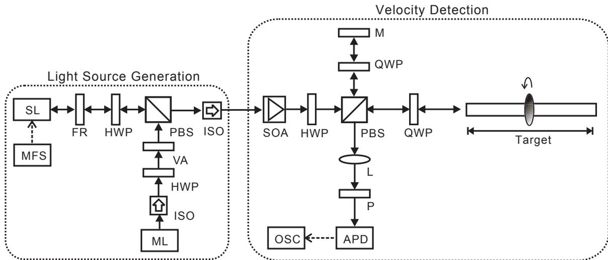
**Figure 1.** Experimental setup of the DF-LDV. ML, master laser; SL, slave laser; ISO, optical isolator; VA, variable attenuator; FR, Faraday rotator; HWP, half wave plate; QWP, quarter wave plate; PBS, polarizing beam splitter; L, lens; M, mirror; P, polarizer; SOA, semiconductor optical amplifier; APD, avalanche photodetector; MFS, microwave frequency synthesizer; OSC, oscilloscope.
