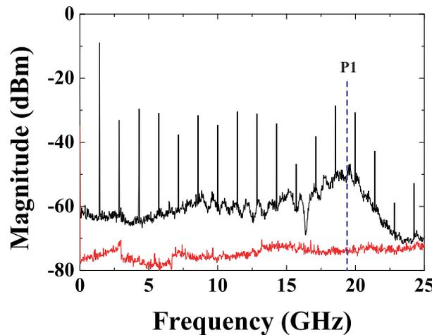
**Figure 5.** Power spectrum of SL chaotic output under combined double phase-locked loop and optical cw injection when  $f_{rep} = 1.425$  GHz. Red curve: background noise level.
