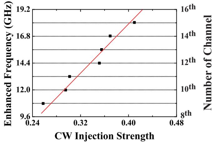
**Figure 4.** Linear tunability between cw injection strength and the selected frequency (channel).
