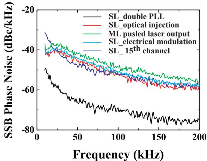
**Figure 6.** SSB phase noise of the 1<sup>st</sup> channels of the pulsed laser output (green) and the SL output when applying optical injection (red), electric modulation (cyan), and double phase-lock loop (black), respectively. Blue curve is the SSB noise of the secondary (15<sup>th</sup>) channel.
