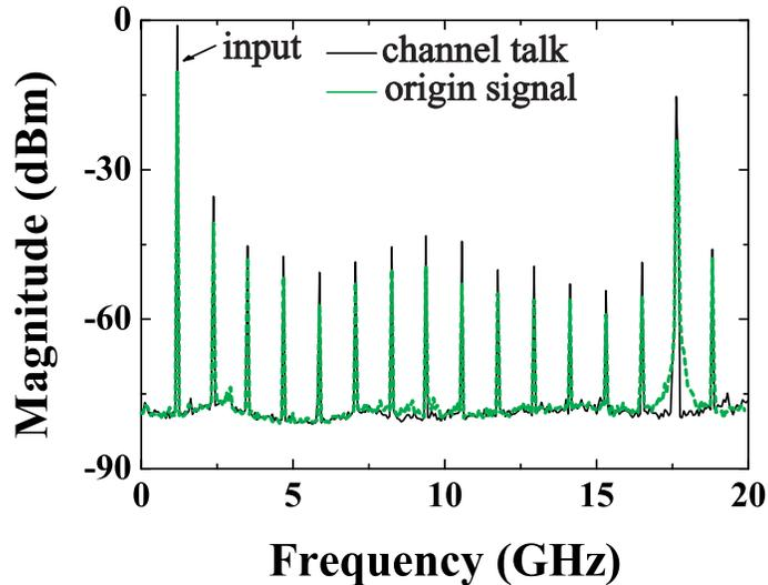
**Figure 7.** Power spectrum of the SL output subject to both double phase-locked technique and optical cw injection (green) and the spectrum after introducing a sinusoidal signal at the 1<sup>st</sup> (main) channel (black).
