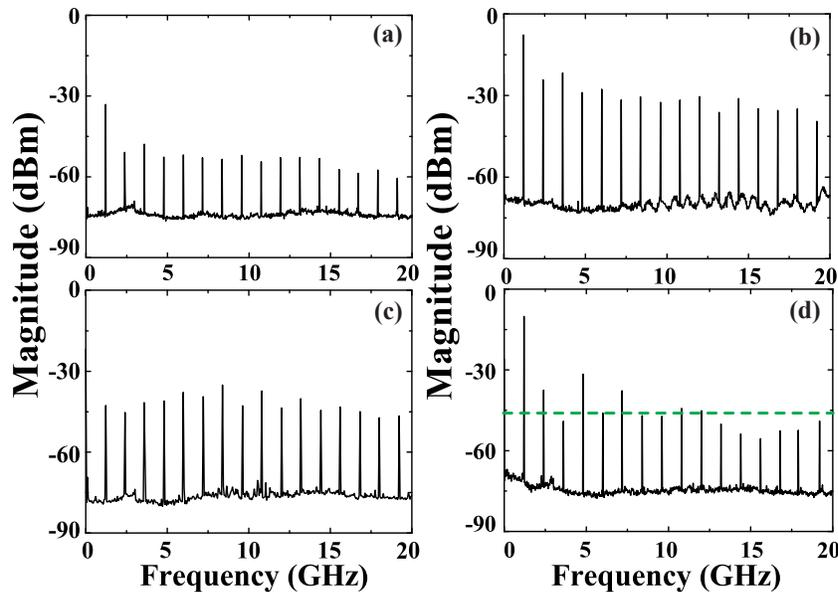
**Figure 2.** Power spectra of (a) the ML output generated by optoelectronic feedback and the SL output when subjected to (b) electric modulation, (c) optical injection, and (d) both electric modulation and optical injection from the ML output. Dashed line: average magnitude.
