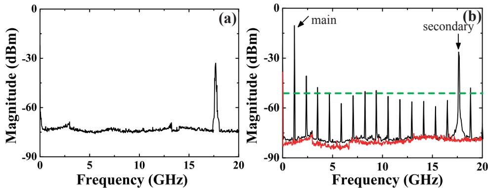
**Figure 3.** Power spectra of the SL output (a) under optical cw injection and (b) subject to both double phase-locked technique and optical cw injection. Dashed line: average magnitude. Red curve: background noise level.
