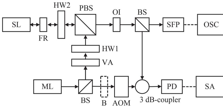
Figure 3. Schematic diagram of the experimental setup. FR: Faraday rotator; HW: half-wave plate; PBS: polarizing beamsplitter; OI: optical isolator; BS: beamsplitter; SFP: scanning Fabry-Perot interferometer; OSC: oscilloscope; PD: photodiode; SA: spectrum analyzer; VA: variable attenuator; AOM: acoustooptic modulator; B: beam block.
