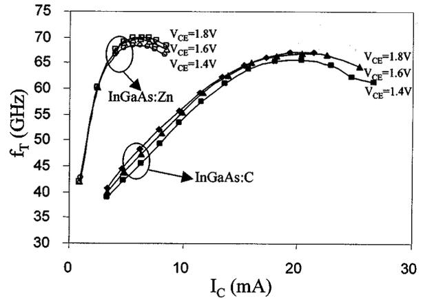
Fig. 6. Dependence of  $f_T$  on dc bias for  $1 \times 10 \mu\text{m}^2$  carbon-doped and zinc-doped InP/InGaAs HBTs.
