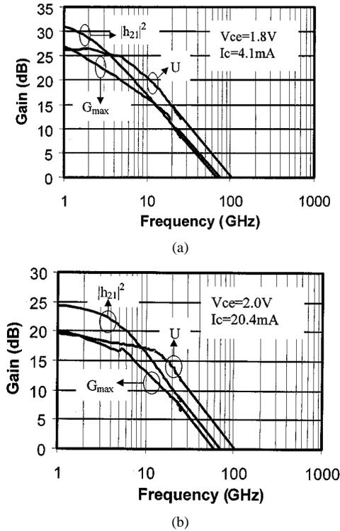
Fig. 5. (a) High-frequency performance of a  $1 \times 10 \mu\text{m}^2$  zinc-doped InP/InGaAs HBT at  $V_{ce} = 1.8 \text{ V}$  and  $I_c = 4.1 \text{ mA}$  and (b) high-frequency performance of a  $1 \times 10 \mu\text{m}^2$  carbon-doped InP/InGaAs HBT at  $V_{ce} = 2.0 \text{ V}$  and  $I_c = 20.4 \text{ mA}$ .
