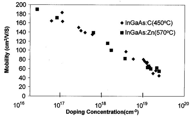
Fig. 4. Hall mobility of carbon-doped InGaAs and zinc-doped InGaAs as a function of doping concentration.
