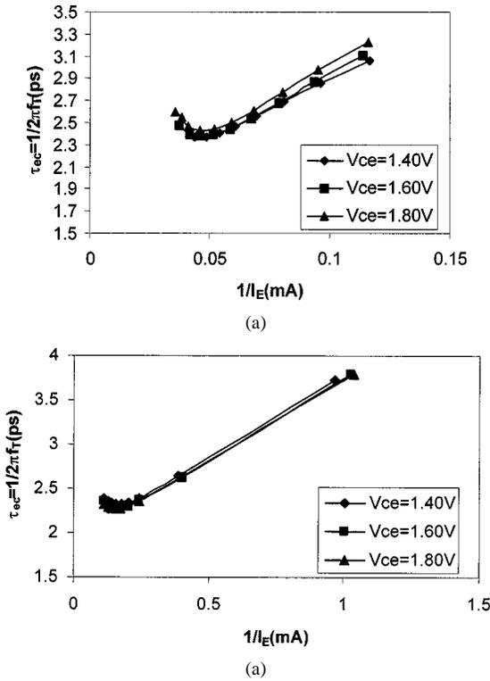
Fig. 7. (a) Plot of  $\tau_{ec}$  versus  $1/I_E$  for  $1 \times 10 \mu\text{m}^2$  carbon-doped InP/InGaAs HBTs and (b) plot of  $\tau_{ec}$  versus  $1/I_E$  for  $1 \times 10 \mu\text{m}^2$  zinc-doped InP/InGaAs HBTs.
