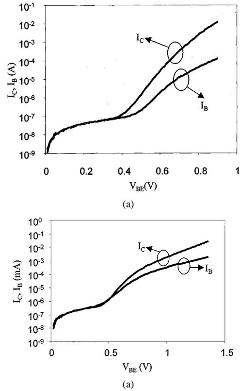
Fig. 2. (a) Gummel plot of  $1 \times 10^4 \mu\text{m}^2$  zinc-doped InP/InGaAs HBT and (b) Gummel plot of  $1 \times 10^4 \mu\text{m}^2$  carbon-doped InP/InGaAs HBT.
