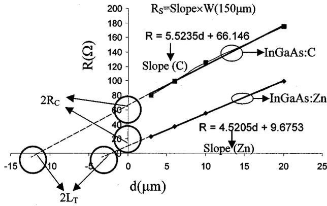
Fig. 3. Plot of total resistance as a function of TLM pad gap size for carbon-doped and zinc-doped InP/InGaAs HBTs.
