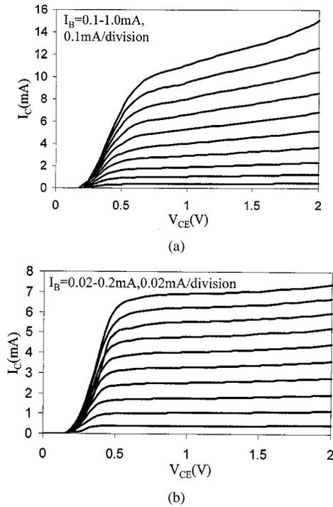
Fig. 1. (a) DC characteristics of  $1 \times 10^4 \mu\text{m}^2$  carbon-doped InP/InGaAs HBT and (b) DC characteristics of  $1 \times 10^4 \mu\text{m}^2$  zinc-doped InP/InGaAs HBT.
