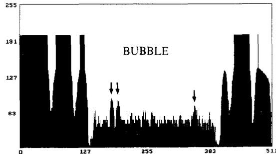
Fig.5 Image of a copper made medal to show the hiding bubbles; the gray level trace along a scanned line is to indicate the locations of the defects.
