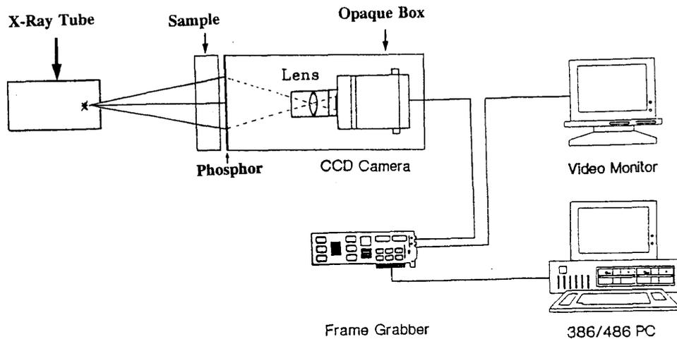
Fig.1 Sketch of the system hardware arrangement
