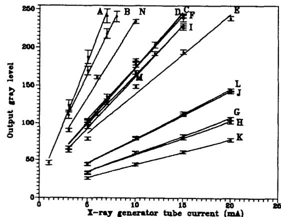
Fig.2 Light output of phosphor screens
