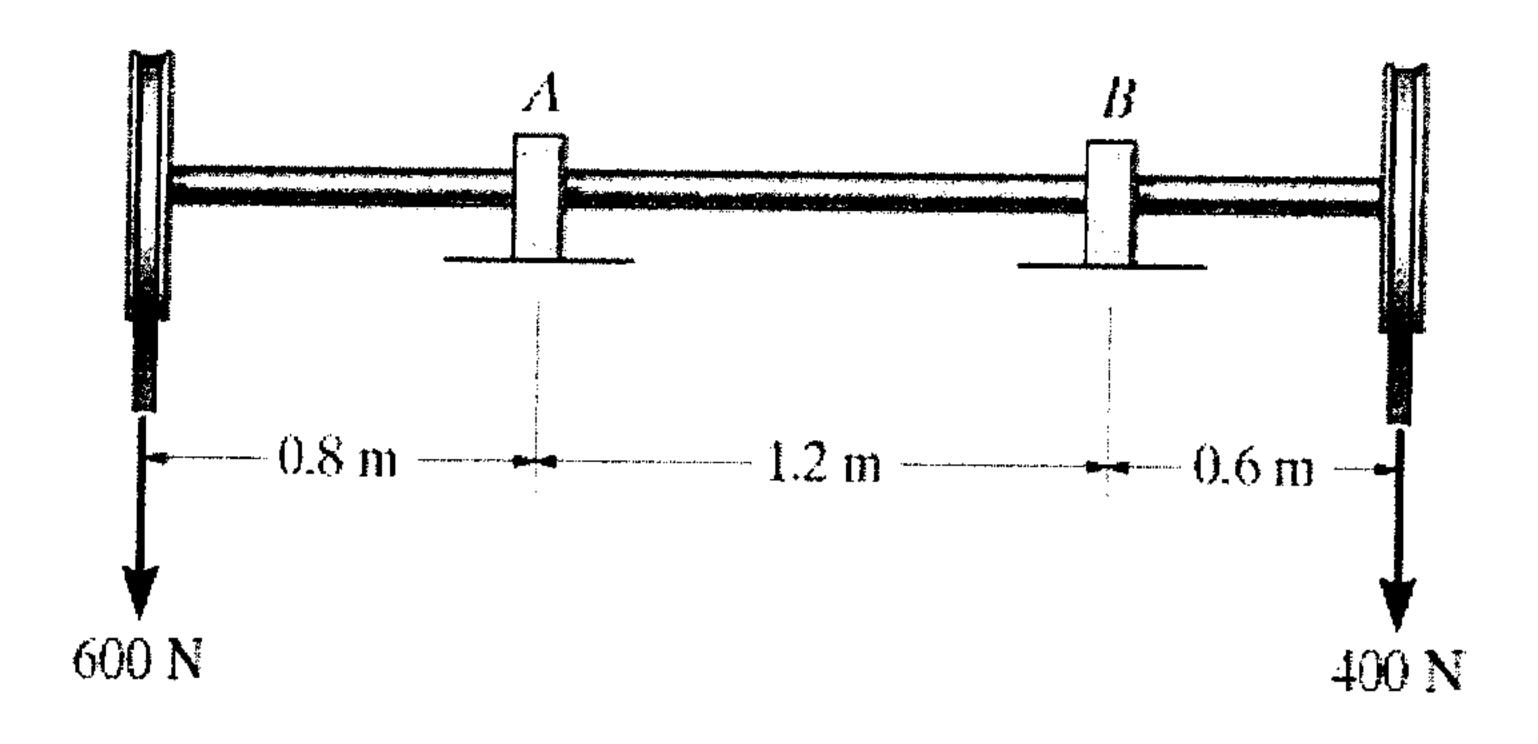
To figure out the proper diameter of the shaft, please draw shear force and moment diagrams in for the shaft as function of shaft's longitudinal axis then complete the following questions.
