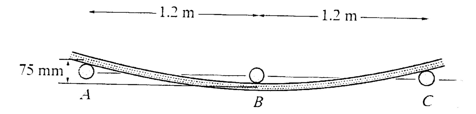
Suppose the centre post B provides force P acting toward the board, to complete the following two questions, you may want to draw free body diagram of the entire system to figure reaction loads on the board by posts A and B, followed by sectioning the beam and using free body diagram and equilibrium equations to figure internal bending moment, shear force, and equation describing elastic curve of the board. From your calculation,
