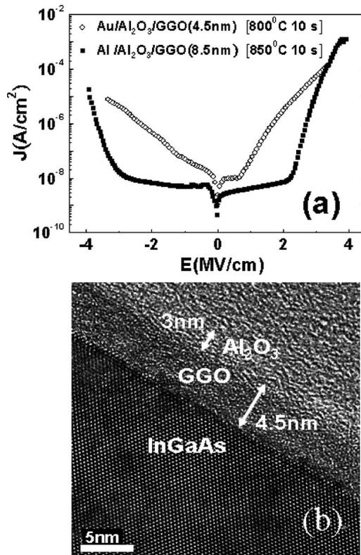
FIG. 3. (a) Leakage current density ( $J$ ) for 4.5 and 8.5 nm samples, subjected to RTA 800 °C 10 s, and 850 °C 10 s under N<sub>2</sub>, respectively. (b) Cross-sectional HRTEM image of the 4.5 nm sample in (a).
