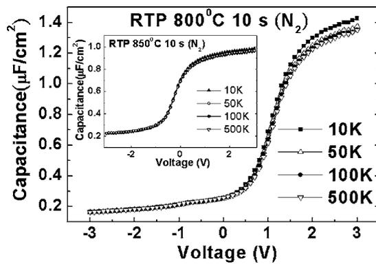
FIG. 1.  $C$ - $V$  characteristics for an  $\text{Al}_2\text{O}_3(3 \text{ nm})/\text{GGO}(4.5 \text{ nm})/\text{In}_{0.2}\text{Ga}_{0.8}\text{As}/\text{GaAs}$  MOS diode RTA to  $800^\circ\text{C}$  with the Au gate deposited afterwards. The inset shows  $C$ - $V$  characteristics of another  $8.5 \text{ nm}$  sample, which was RTA to  $850^\circ\text{C}$  with the Al gate. The capacitor area is  $7.85 \times 10^{-5} \text{ cm}^2$ .
