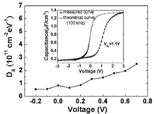
FIG. 2. Distribution of  $D_{\text{it}}$  ( $4.5 \text{ nm}$  sample of Fig. 1) near the midgap measured using the high frequency conductance method. Small flatband voltage and differences between the measured and theoretical  $C$ - $V$  curve at  $100 \text{ kHz}$  are shown in the inset.
