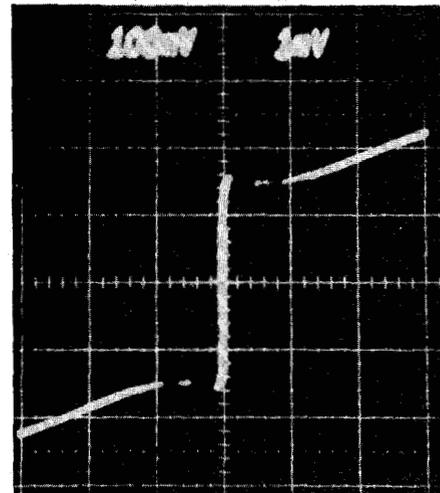
Figure 1 Current-voltage characteristics of a Pb VTB at  $T \leq 2$ K. Vertical scale: 10mA/div., horizontal scale: 1mV/div.
