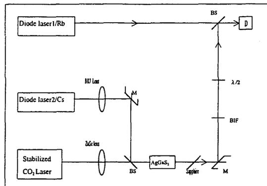
Fig.1 Experimental setup for the absolute frequency measurement of the Cs D<sub>2</sub> line at 852nm. BS: beam splitter; Here, M: mirror; BIF: bandpass interference filter; D: avalanche photodiode. The outputs of all lasers are linearly polarized vertically and the sum-frequency radiation is polarized horizontally.
