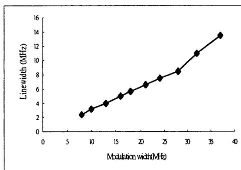
Fig. 3 Modulation broadening of the d-f crossover line. Here, pump power: 70  $\mu$ W; probe power: 8  $\mu$ W; temperature: 11  $^{\circ}$ C; modulation frequency: 9.8 kHz.
