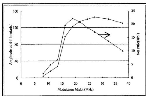
Fig. 2 Signal strength and S/N ratio of the d-f crossover line vs. modulation width. Here, pump power: 70  $\mu$ W; probe power: 8  $\mu$ W; temperature: 11  $^{\circ}$ C; modulation frequency: 9.8 kHz.
