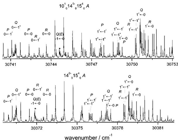
FIG. 3. Portion of spectra in ranges 30 740–30 753  $\text{cm}^{-1}$  (upper) and 30 368–30 382  $\text{cm}^{-1}$  (lower) for  $10_0^1 14_0^0 15_0^4$  and  $14_0^0 15_0^4$ , respectively, showing similar rotational structures. Transitions  $K'-K''$  and  $\Delta J = -1, 0 + 1$  for P, Q, and R branches are indicated. Symbol \* denotes  $14_0^0 + 15_0^4(E)$  and  $10_0^1 14_0^0 + 15_0^4(E)$  for the lower and upper spectrum, respectively.
