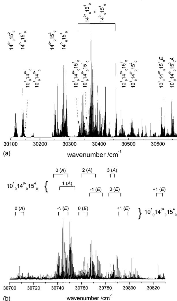
FIG. 1. Spectra and vibrational assignments for  $\tilde{A}^1 A''$ – $\tilde{X}^1 A'$  of CH<sub>3</sub>CHO for excitation in regions (a) 30 100–30 660 cm<sup>-1</sup> and (b) 30 700–30 830 cm<sup>-1</sup> showing the progressions  $10_0^1 14_0^+ 15_0^n$  and  $10_0^1 14_0^- 15_0^n$  with  $n = 0-4$ . In (b) the  $K'$  quantum number is shown.
