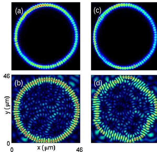
Fig. 2. Near field intensity distributions on the surface of aperture of our micro-structured VCSEL at different injection currents. Experimental data: (a) 19mA and (c) 20.5mA; corresponding simulation results (b) and (d) with the same azimuthal number, 41.
