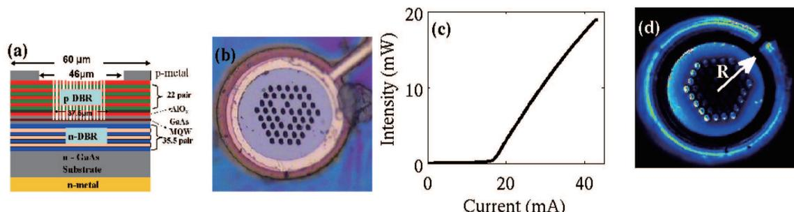
Fig. 1. (a) The schematic diagram, (b) corresponding SEM image of the surface micro-structure, and (c) L-I curve for our VCSEL. (d) The near-field collected spontaneous emission patterns operated below the threshold current.
