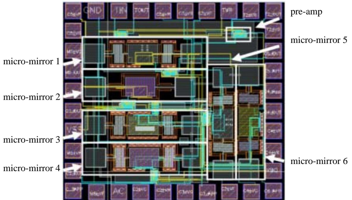
**Figure 2: CMOS layout showing six integrated mirror designs, and one test pre-amp.**
