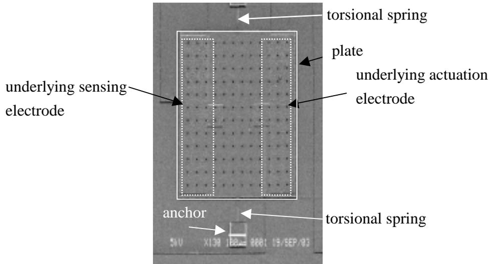
**Figure 1: SEM illustrating the top view of the fabricated polysilicon micro-mirror.**
