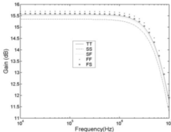
**Figure 4: Corner analysis of the pre-amplifier magnitude response illustrating the possible gain variations.**
