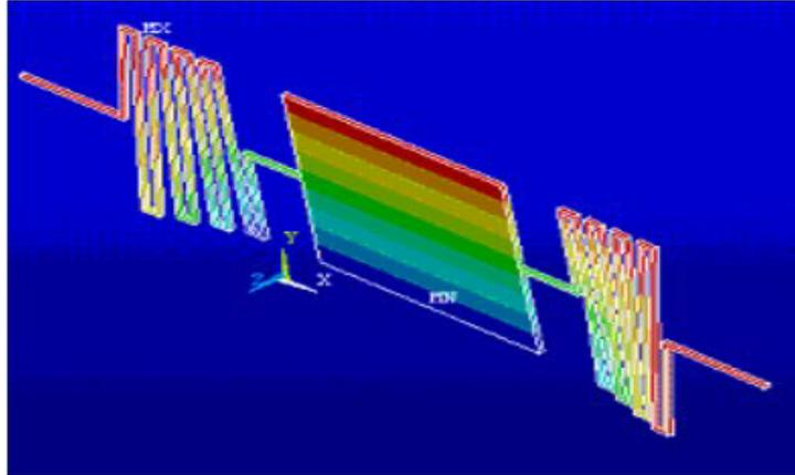
**Figure 3: Finite-element analysis of CMOS-MEMS micro-mirror.**
