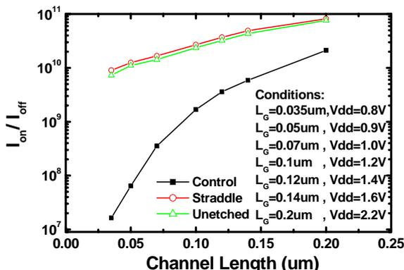
Fig.5 Straddle-gate transistors have higher  $I_{on}/I_{off}$  ratios as device scales down.
