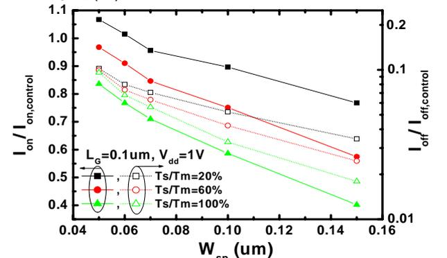
Fig.9 The  $I_{on}$  and  $I_{off}$  characteristics of straddle-gate transistors with  $T_s/T_m$ (%) vs.  $W_{sp}$ .
