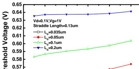
Fig.6  $V_{th}$  of straddle-gate transistors with different straddle oxide  $T_s/T_m$  ratios while  $T_m$  (main gate oxide thickness) is fixed.
