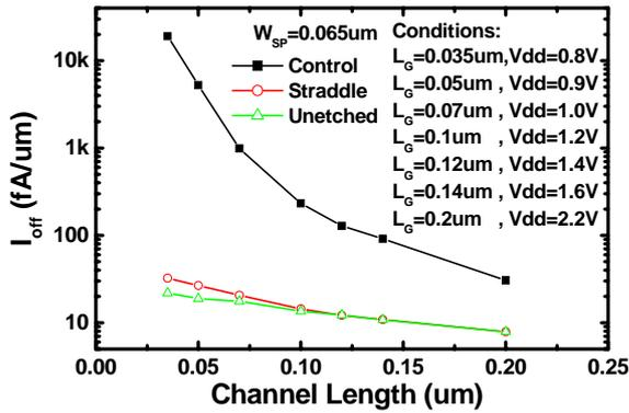
Fig.3 The off-state current of control device is 1~3 order higher than the others.
