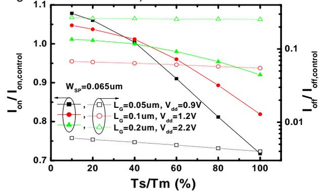
Fig.7 The  $I_{on}$  and  $I_{off}$  characteristics of straddle-gate transistors vs.  $T_s/T_m$ (%).
