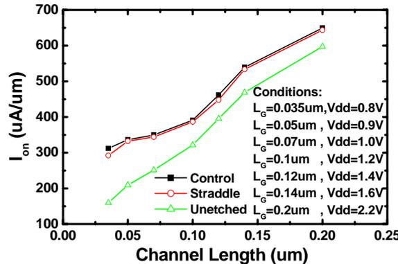
Fig.4 No significant difference is observed between control device and straddle device.
