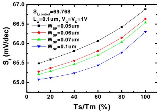
Fig. 10 The thinner the straddle oxide thickness, the lower the sub-threshold slope is.
