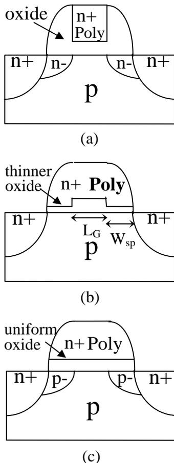
Fig.1 Schematic cross-section of (a)control device, (b)straddle-gate transistors and (c)unetched-gate transistors simulation.
