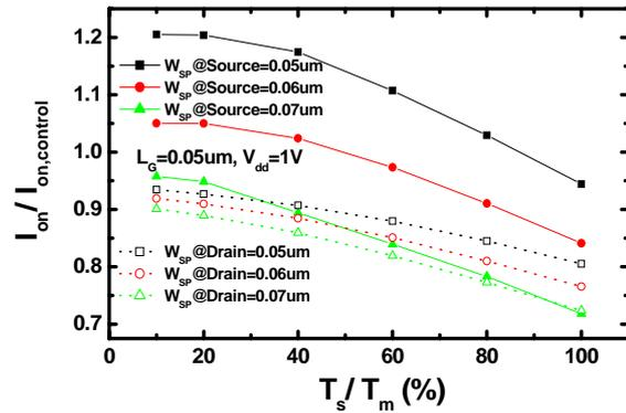
Fig.12 The on-state currents of one-sided straddle-gate transistors.
