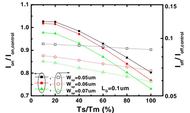
Fig.8 The  $I_{on}$  and  $I_{off}$  characteristics of straddle-gate transistors with different spacer width vs.  $T_s/T_m$ (%).
